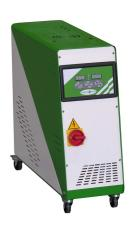
**GREEN BOX** is proud to present the completely restyled TB-S, TB-M and TB-D series of mould temperature controllers. These units are available in water, oil and water/oil versions, all with open tank, reversible pump and with working temperatures up to 90℃ (wate r) or 150℃ (oil).
