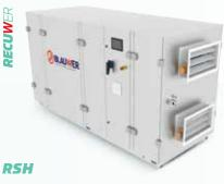
Swimming-pool air handling unit, fully configurable, with high efficency heat recovery, integrated heat pump. Heting capacity 8 - 139 kW. Air flow 1500 - 14000 m3/h
